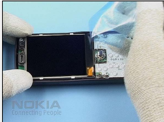
38. After removal of the plastic film check the surface of the DISPLAY for cleanliness.
