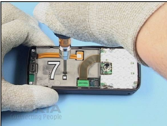
35. Now, tighten the last screw to the correct torque.
