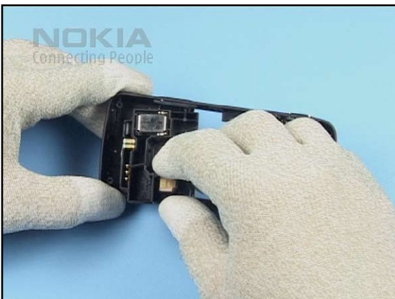
39. ... and remove it from the B-COVER.
