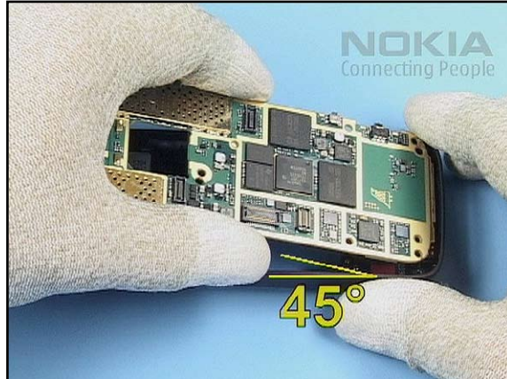
14. Insert the ENGINE MODULE under the shown angle.
