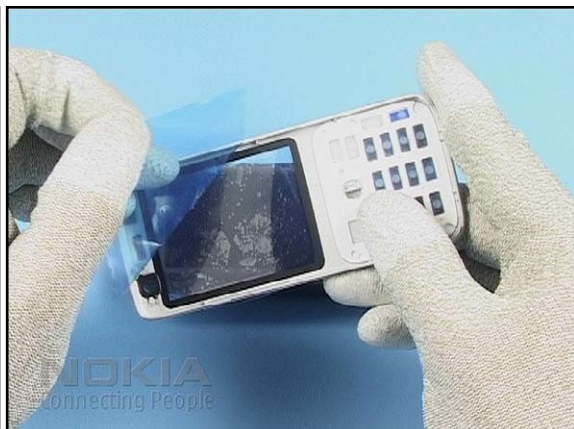
42. Check the window for cleanliness ...
