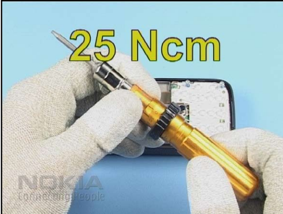
31. Set the torque driver to the torque of 25 Newton centimeter.
