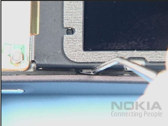
13. Carefully unlock and remove the DISPLAY SHIELD by using the dental tool.
