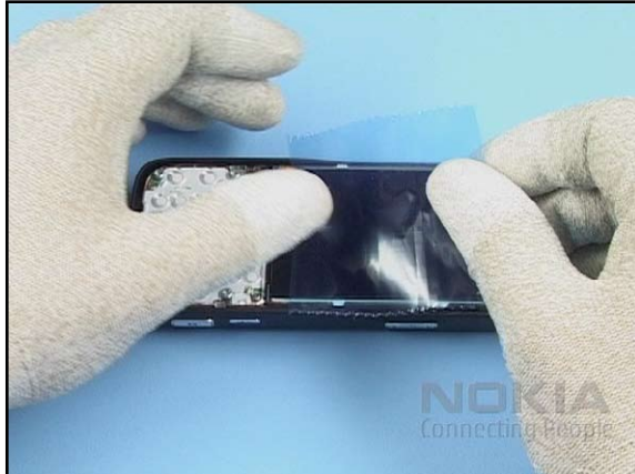
14. Cover the DISPLAY with a protective film.
