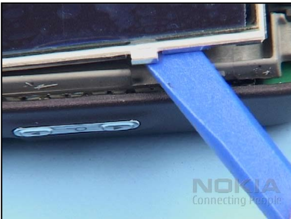
15. Gently lift out the DISPLAY with the SS-93 from the UI FRAME...
