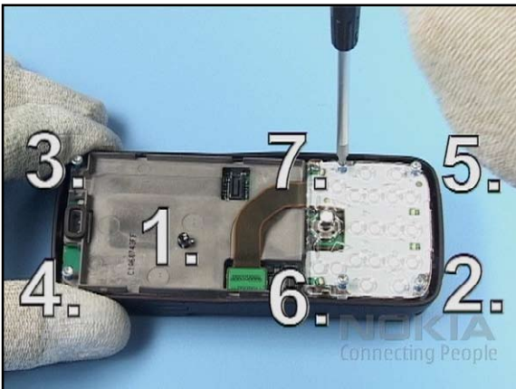
21. Undo the screws in the order shown.
