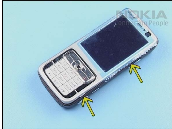
8. Slide the SRT-6 along the marked edges to unlock the snaps.
