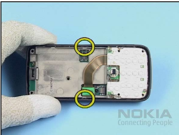
23. The UI FRAME is attached with two snaps to the B-COVER.
