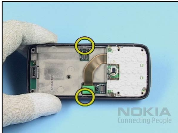
28. Put the UI FRAME into the B-COVER and press it into place.
