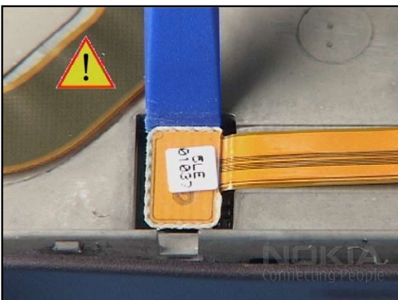
17. Open the FRONT CAMERA connector.
