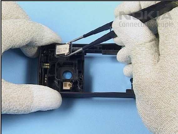
13. Insert the IHF SPEAKER paying attention to its spring contacts.
