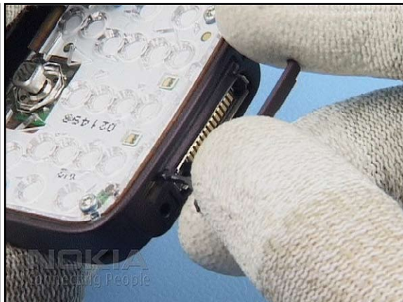
40. Insert the SD DOOR but do not close it yet.
