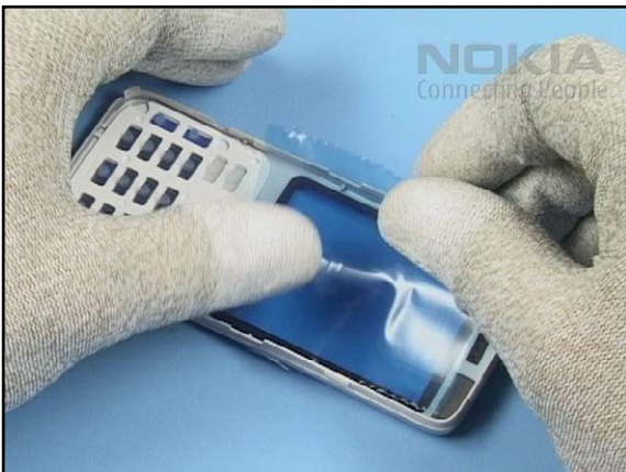
11. Remember to protect the inner side of the window with a protective film.
